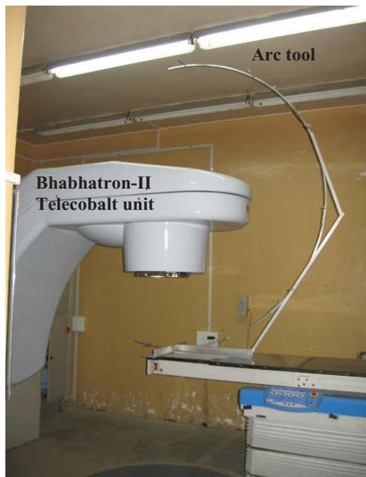
Fig. 1 Photograph showing experimental arrangement used for leakage measurement from source head of Bhabhatron-II telecobalt unit (couch angle is  $0^\circ$  in this case).
