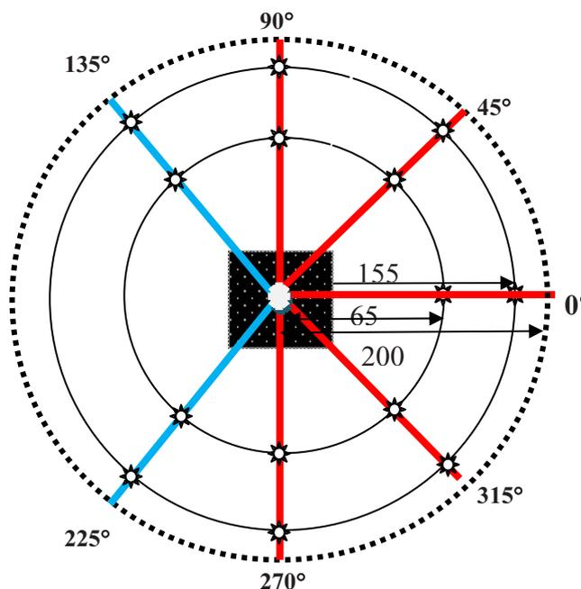
Fig. 2 Schematic diagram showing measurements positions in patient plane at 65 and 155 cm from the radiation beam axis. Black shaded region indicates area under the collimator zone. Indicated angular positions are the couch positions.
